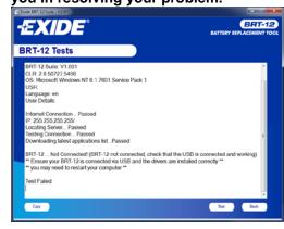
7. Connect your BRT-12 as per the instructions within the BRT-12 update suite. Connect mini USB to BRT-12 and USB to PC. Refer to the 'BRT-12 Update Procedure' for more information.
